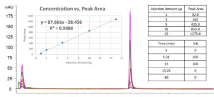
Column : Sepax BioService Affinity HSA 2.1 x 50 mm PEEK (P/N: 272101P-2105); Mobile phase A: 20mM phosphate,150mM NaCl, pH 7.5; B: 0.1 M Glycine, pH 2.5; Flow rate: 0.5 mL/min; Detector: 280 nm; Column temperature: 25  $^{\circ}$  C
